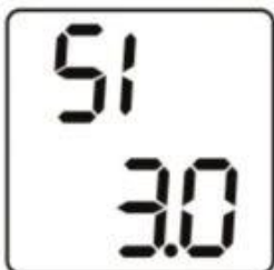
if over-current fault last 3s, output load switch off
