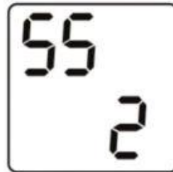
Delay 2s in load switch on after input power on
