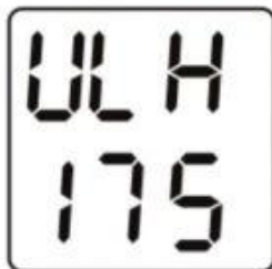
175V under voltage recovery
