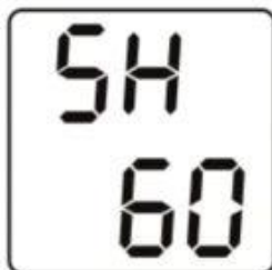
Delay 60s for recovery load after output load switch off protection
