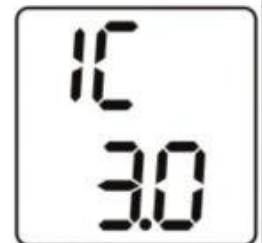
3A Malignant load protection (Pure Resistive Load limit)
