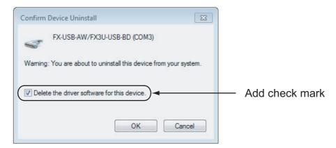
Add a check mark to [ Delete the driver software for this device. ], and click [ OK ]. The USB Serial Port software is uninstalled.
