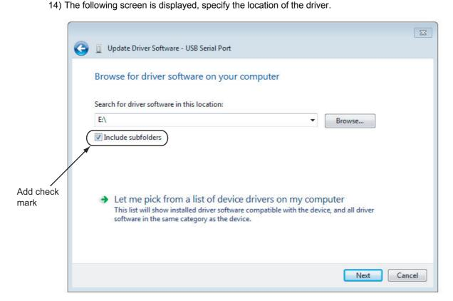
Add a check mark to [Include subfolders]. Insert the CD-ROM that has the driver software into the personal computer. Select the CD-ROM drive, and click [Next].
