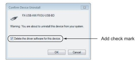
Add a check mark to [ Delete the driver software for this device. ], and click [ OK ]. The USB driver is uninstalled.
